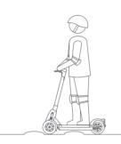
Keep your speed between 5--10 km/h when you ride through speed bumps, elevator door stills, bumpy roads or other uneven surfaces. Slightly bend your knee to better adjust mentioned surfaces.
