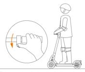
3. Put your other foot on the footboard to keep both feet stable. Press the throttle on the right hand to speed up when you are balanced. Note, for your safety, the motor will not engage until the KickScooter is no less than 1.9 mph (3 km/h).
