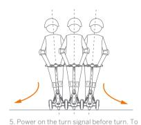
turn, shift your body weight and turn the handle slightly. Power off when turn finished.
